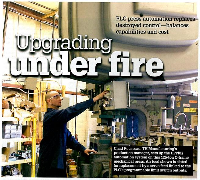
ooking a press control under deadline pressure isn't the ideal circumstance for upgrading a stamping operation. But a fire in a 1950s-era hard-wired relay system for a 125-ton C-frame mechanical press sent TH Manufacturing Co. on an urgent search for replacement technology.
